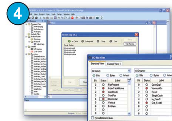
4 Run the application from the EPSON RC+ Run Window or set to have GUI come up automatically. You can also bring up RC+ dialogs like the I/O monitor shown here.
